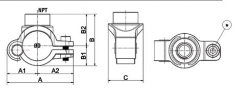
Note: Requires hole saw bit to drill pipe. 1/2" = 14 mm hole saw drill bit (ANK0043). 3/4" = 19 mm hole saw drill bit (ANK0143). 1" = 24 mm hole saw bit, includes Arbor and Pilot, (ANK0342). ANK0243 Drill arbor and pilot bit also required
