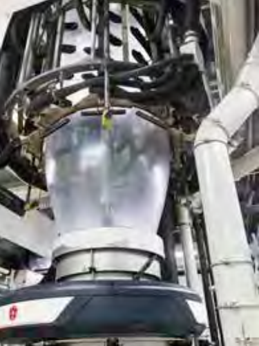
Image, left: Huge sheets of foil are produced inside these towering extruders. Image, right: The new compressed air station is arranged on two levels to save space.
